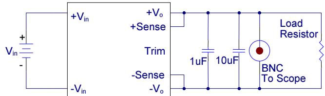
Output ripple and noise is measured with 1.0uF ceramic and 10uF solid tantalum capacitors across the output.
